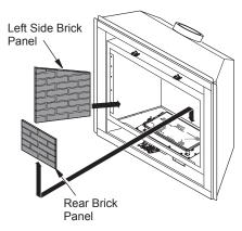
Figure 44 - Installing Rear Brick Panel
